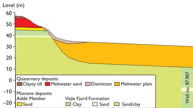
Fig. 7. Conceptual geological model along the motorway alignment.
