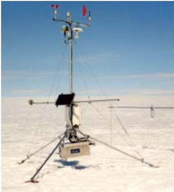
Fig. 2. The new one-mast design of the automatic mass-balance stations installed in the field in May 2001; height *c.* 2.2 m (AMS 71). The gallows with the sonic ranger for surface height measurements can be seen to the right.
